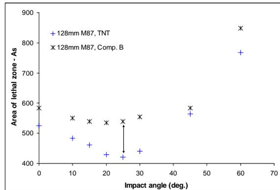
**Fig 16.** Influence of explosive type used on projectile terminal effectiveness (rocket projectile warheads)
