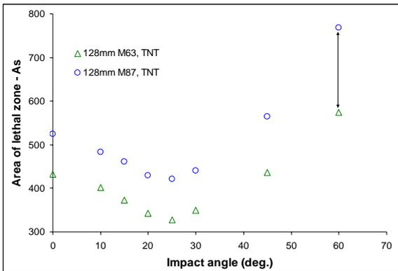
**Fig 15.** Influence of projectile design on terminal effectiveness (rocket projectile warheads)
