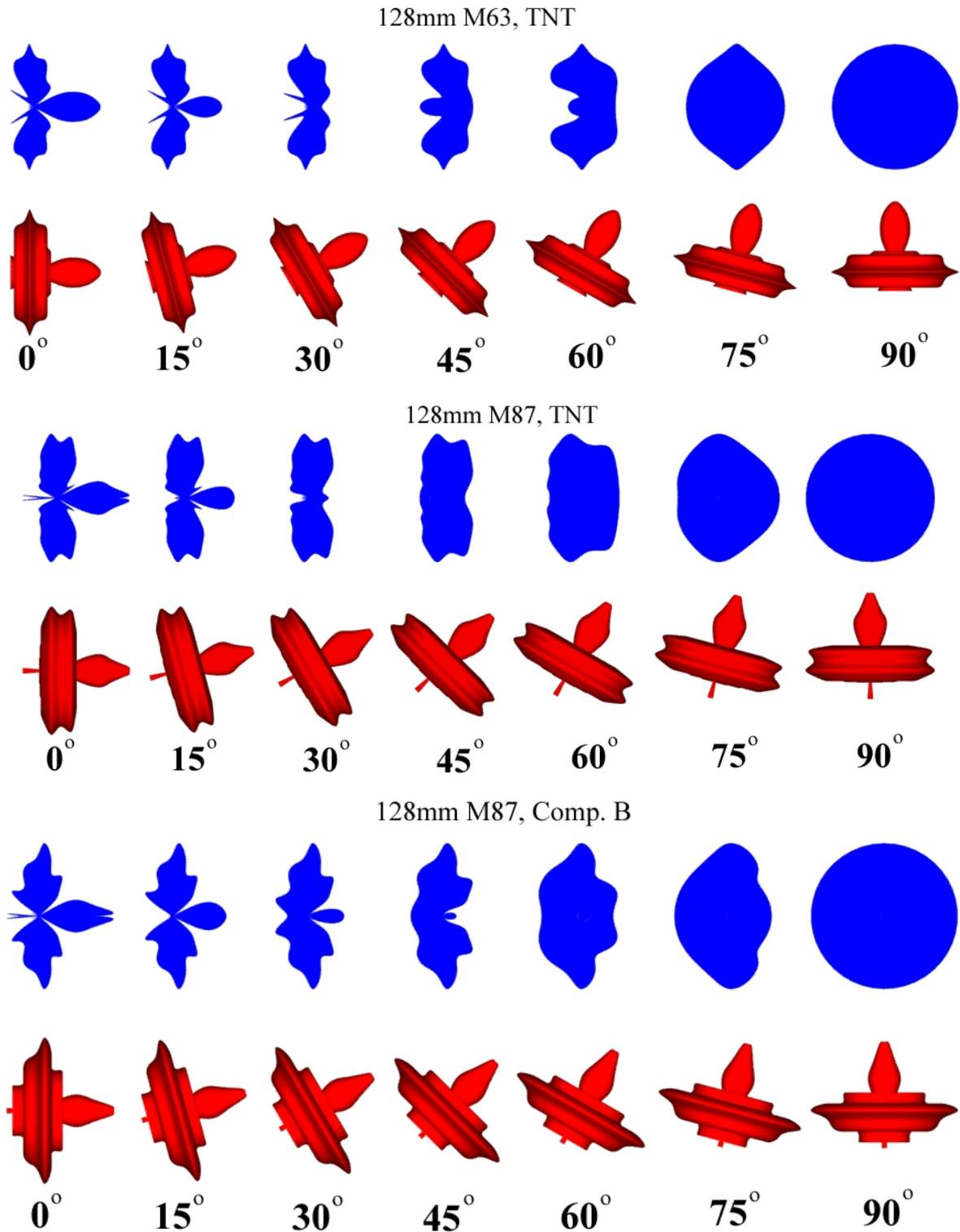
**Fig 13.** 2D lethal zones for different impact angles of tested rocket projectile warheads 128mm
