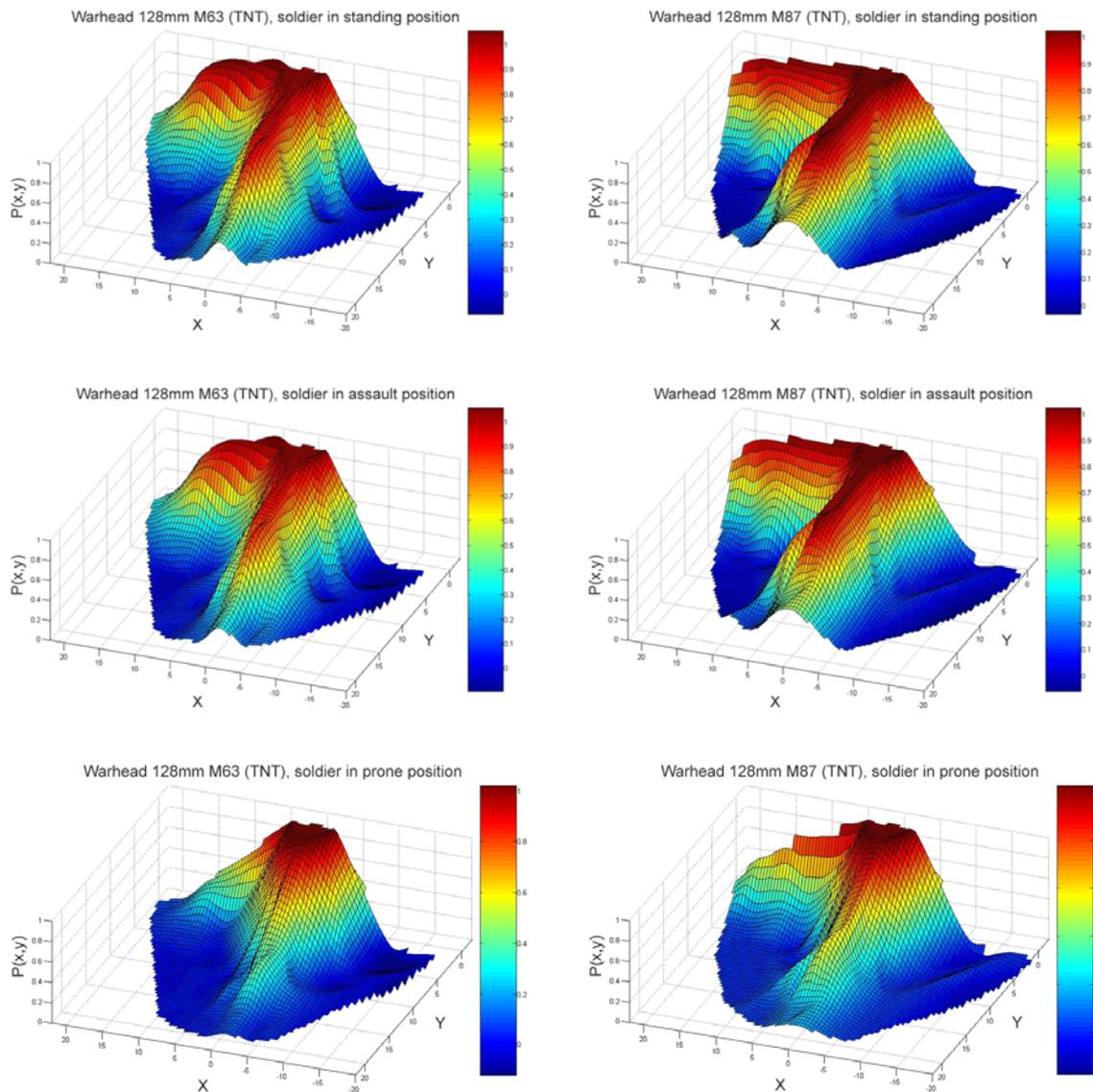
**Fig 10.** Incapacitation probability as a function of three different presented area of the soldier, for rocket projectile warheads 128mm M63 and 128mm M87
