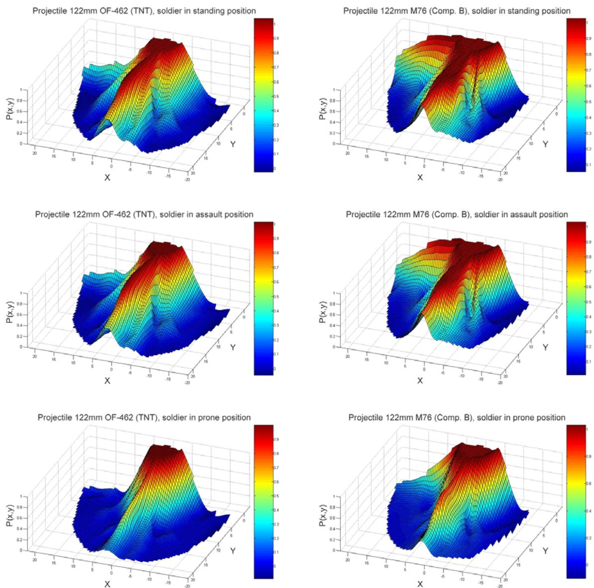
**Fig 9.** Incapacitation probability as a function of three different presented area of the soldier, for projectiles 122mm OF-462 and 122mm M76
