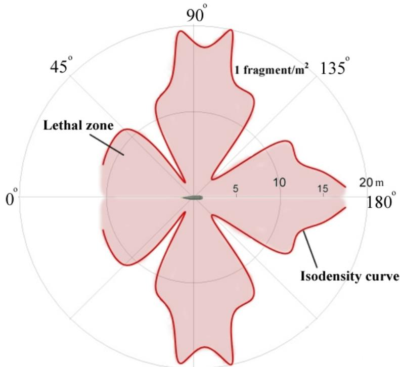
**Fig 3.** Isodensity curve and lethal zone for 0° projectile impact angle<sup>[9]</sup>
