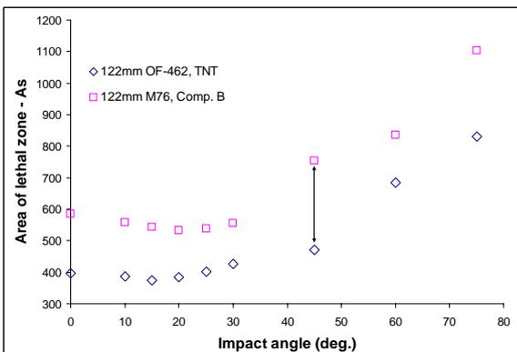
**Fig 17.** Influence of projectile design and explosive type on terminal effectiveness (artill. projectiles)
