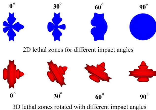
**Fig 7.** 2D and 3D Lethal zones for different projectile impact angle [2]
