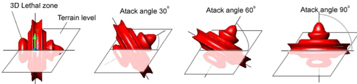
**Fig 6.** 3D model of warhead lethal zone for different projectile angle of attack [2]
