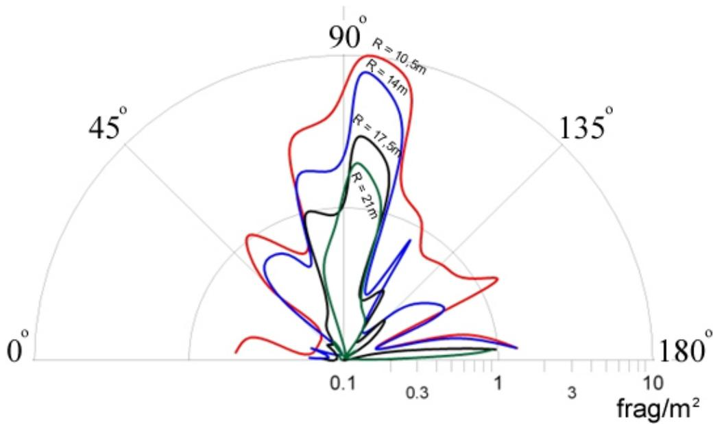
**Fig 2.** Efficient fragment density vs polar angle for different radiuses <sup>[9]</sup>
