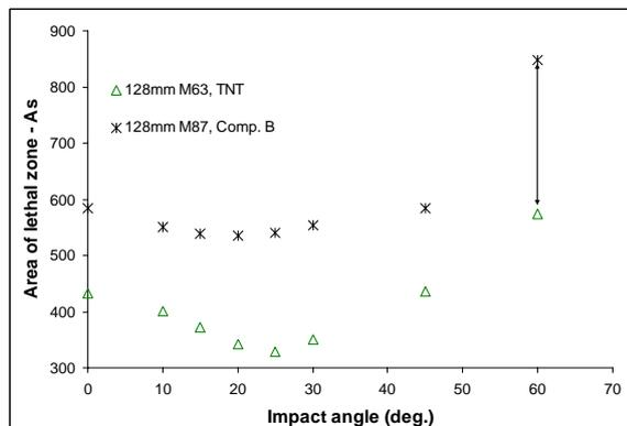
**Fig 18.** Influence of projectile design and explosive type on terminal effectiveness (rocket warheads)
