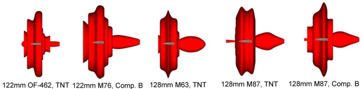
**Fig 11.** 3D lethal zones for tested projectiles
