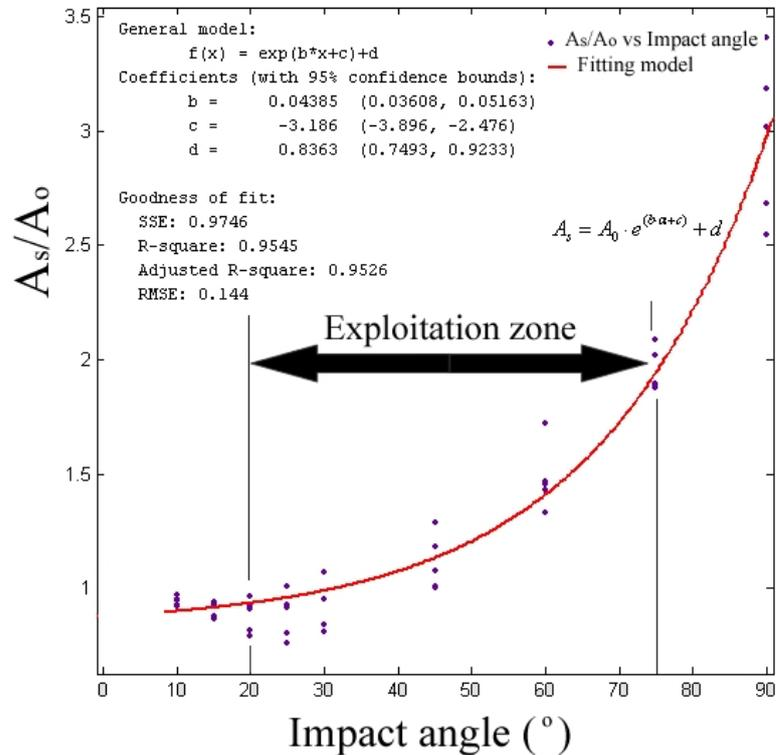
**Fig 14.** Approximation functions of lethal zone area vs projectile impact angle for tested artillery projectiles and rocket projectile warheads
