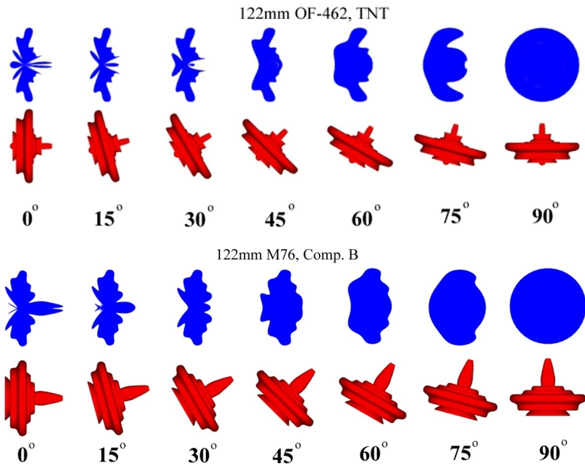
**Fig 12.** 2D lethal zones for different impact angles of artillery projectiles 122mm
