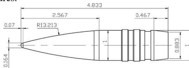
**Figure 8:** Projectile 30 mm PGU-14/B API (dimensions in calibers)
