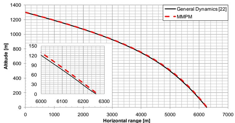
**Figure 11:** Comparison of trajectory based on simulation with MPMM model and reference [22].
