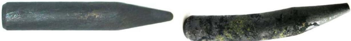
**Figure 19:** Deplete uranium penetrators of ammunition PGU-14/B
