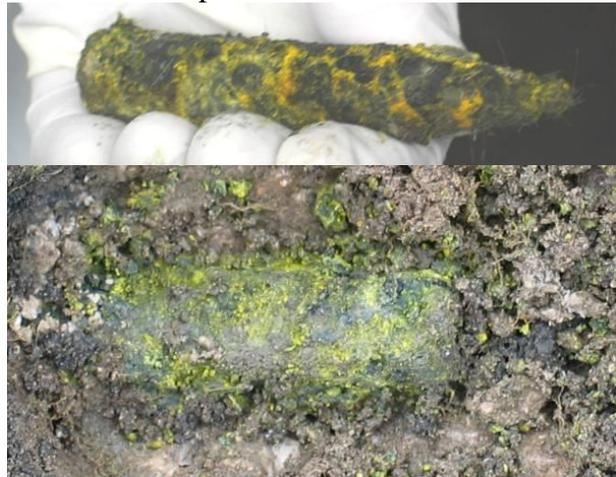
**Figure 18:** Oxidations of penetrators of ammunition PGU-14/B (Military Repair Facility)
