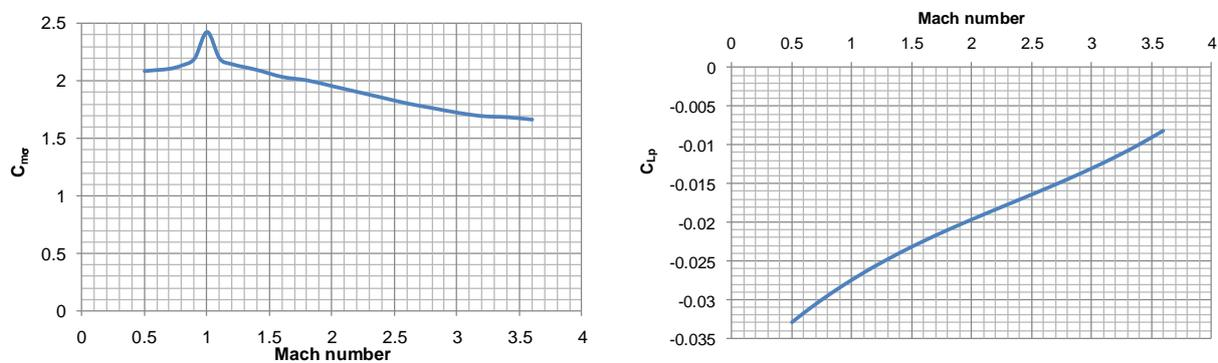
**Figure 10:** Aerodynamic coefficients: pitching moment and axial (left) damping moment (right).
