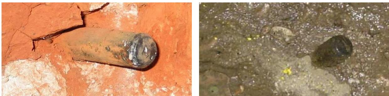
**Figure 20:** Impact penetrator in brick and concrete target
